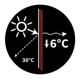
During summertime FRCertified curtains have an impact on the solar energy transmission factor (g) and keep it as low as possible. The solar energy transmission factor when hanging FrCertified curtains can be calculated according to the simplified norm NBN EN 13363-1.
